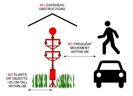
It is not recommended that the BTD sensor is installed on the roof of a tall building as this significantly changes the electric field experienced by the sensor as well as
