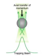
Figure 2: Axial force from refracted beam
