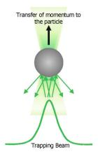
Figure 1: Suspending force from scattered light
