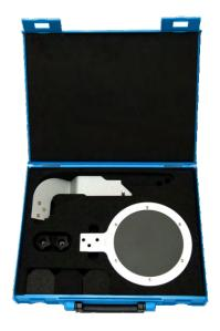
To check the reading accuracy of the VPF series of visibility and present weather sensors
