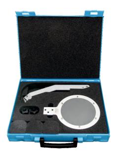
To check the reading accuracy of the SWS and RWS series of visibility and present weather sensors
