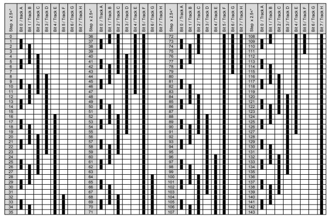
Figure 1: Thies Code table for 8 bit parallel
