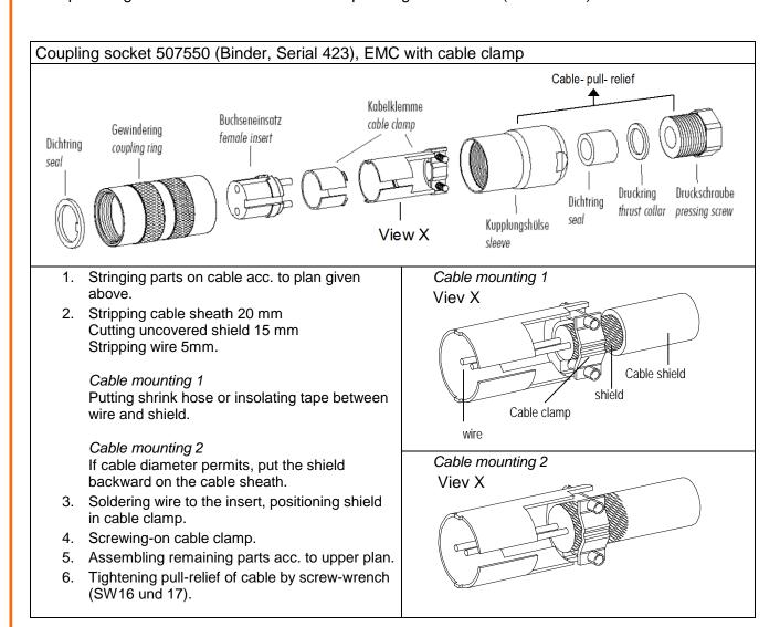
Figure 1: Coupling socket installation
