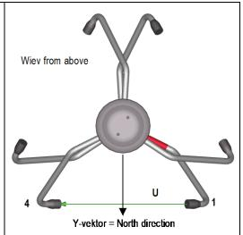
In the bottom of the anemometer stand there is a **north- drilling**. The north- drilling serves for the use of a so-called north- ring with bolt. The north- ring is not included in delivery.
