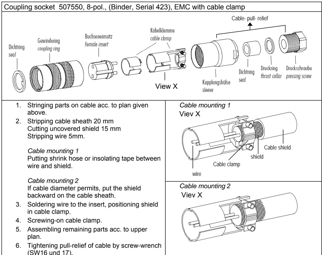
**Figure 1: Connector installation**
