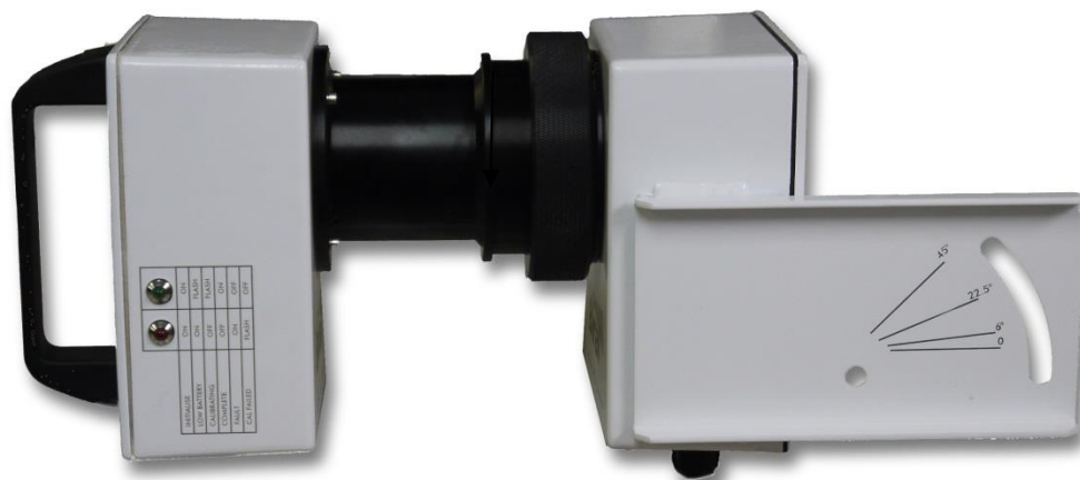
Figure 6: Calibrator connected to ALS-2
