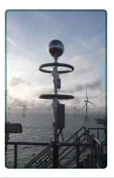
The quasi electrostatic operating principle used by the BTD range allows the sensors to monitor the strength of the local electric field and the presence of charged precipitation, both of which are strong indicators of lightning risk. This allows the BTD range to provide warnings of the risk of an overhead strike even before any lightning has been produced; giving users more time to take the appropriate safety measures ahead of the first strike.
