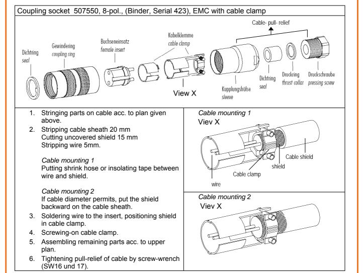
Figure 1: Connector installation
