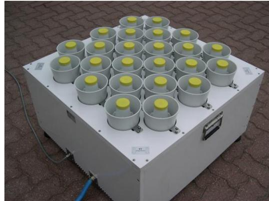
SODAR PCS.2000-24 acoustic shielding (left) and antenna (right)
