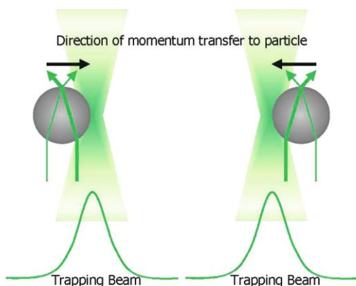
Figure 3: Lateral forces from refracted light
