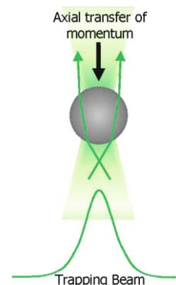
Figure 2: Axial force from refracted beam
