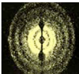
Spatial Scattering Profiles for a Sphere Particle Shape (image kindly provided by The University of Hertfordshire)
