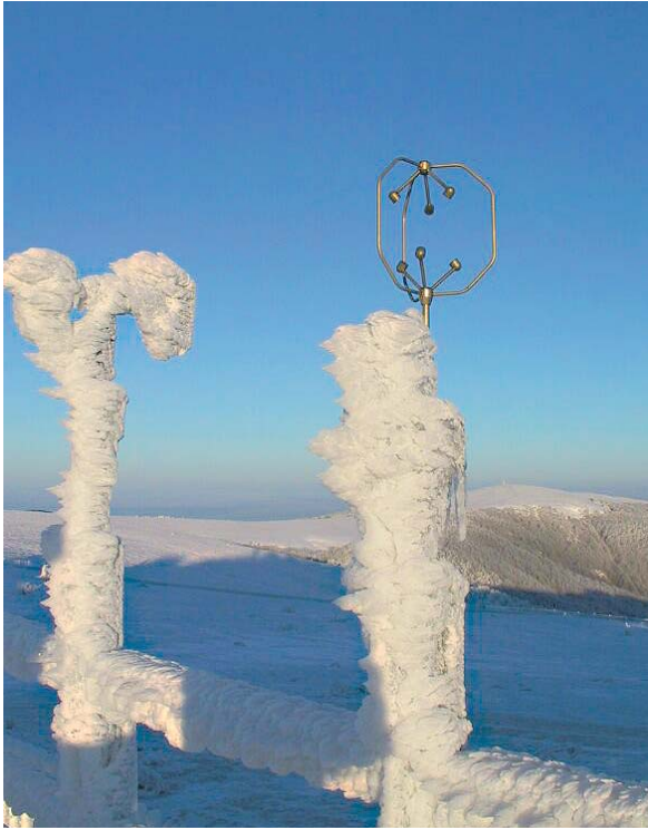
The Metek USA-1 sensor with heating performed well during the recent EUMETNET SWS II study
