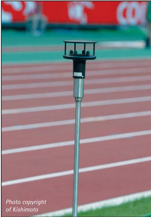
WindSonic anemometer in action as part of the stadium wind measuring system
